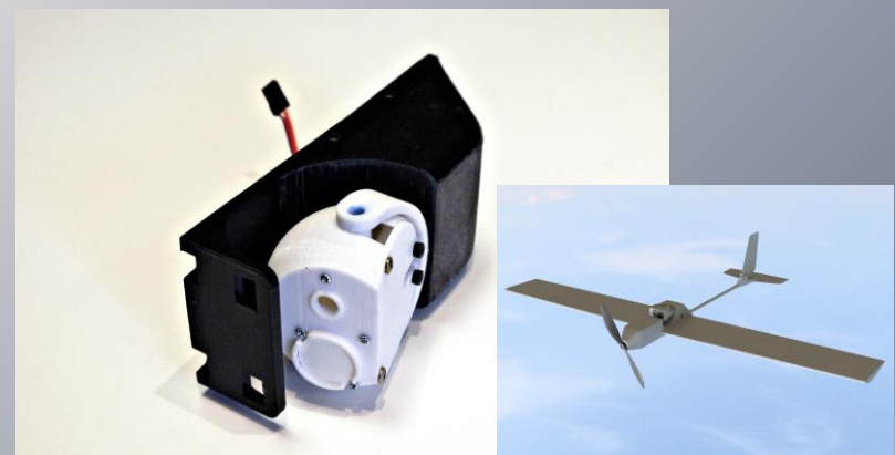
Fixed-wing UAV „Širše“ Roll-Pitch camera positioning module (HW)
